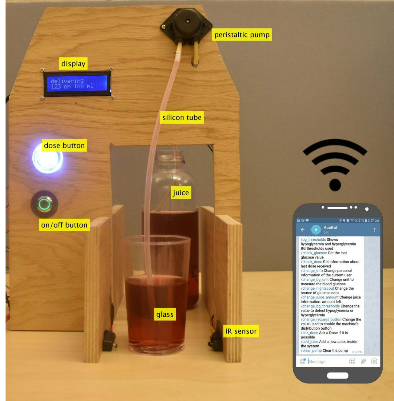
Figure 1: First Prototype, based on communication with Dexcom G4 CGM and the Nightscout solution.
